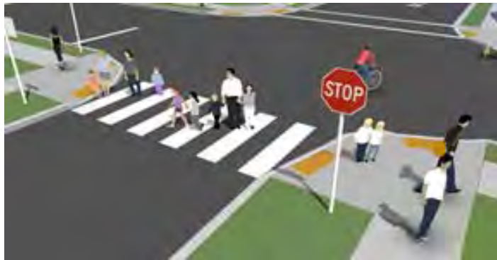
FIGURE 7-12. HIGH VISIBILITY CONTINENTAL STYLE CROSSWALK
